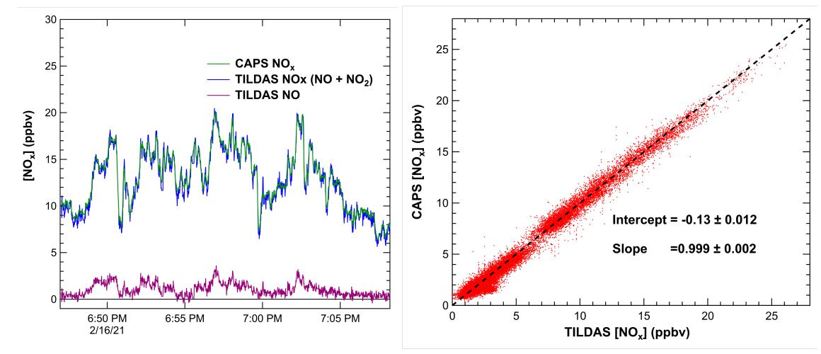
Comparison of 1 second measurements on Aerodyne Mobile Laboratory from CAPS NO<sub>x</sub> and TILDAS NO<sub>x</sub> (NO+NO<sub>2</sub>) monitors.
