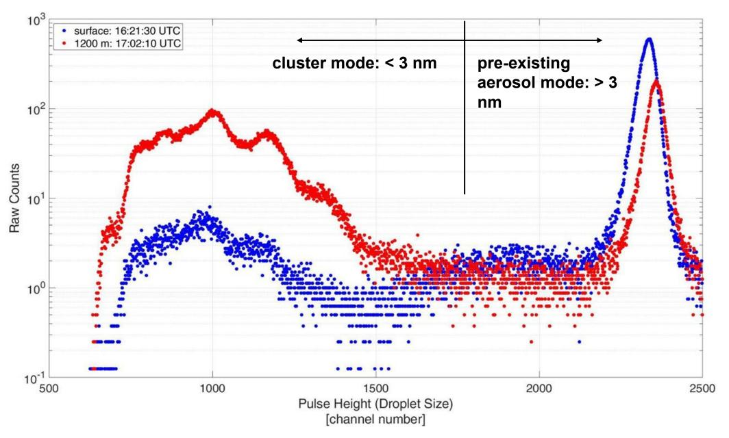
pulse height spectra observed near the surface (16:21:30 UTC) and at 1200 m (17:02:10 UTC).
