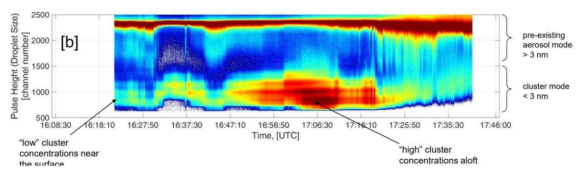
[a] TBS profile altitude as a function of profile time. [b] pulse height contour plot as a function of profile time with preexisting aerosol mode (> 3 nm, > 1500 channel number) and cluster mode (< 3 nm, < 1500 channel number).
