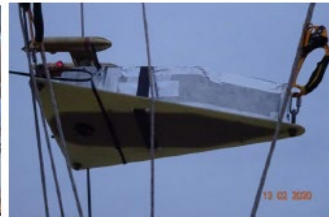
Fig 4b: Gondola suspended on a base plate attached to the tethered balloon system (TBS).
