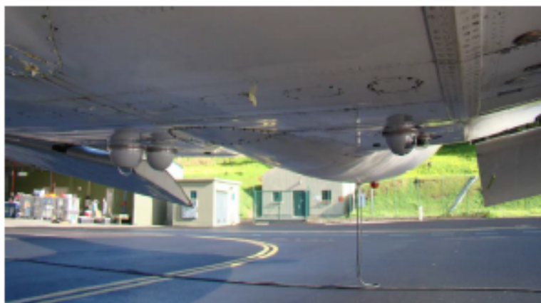
Proposed camera for new AAF (BC-850): Hyperspectral Imager Data: Image cubes at hundreds of wavelength (350-2500 nm)
