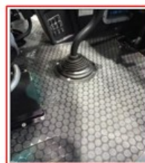
LONSEAL FLOOR Flammability FAR 25.853(a) Friction FAR 25.793(a)
