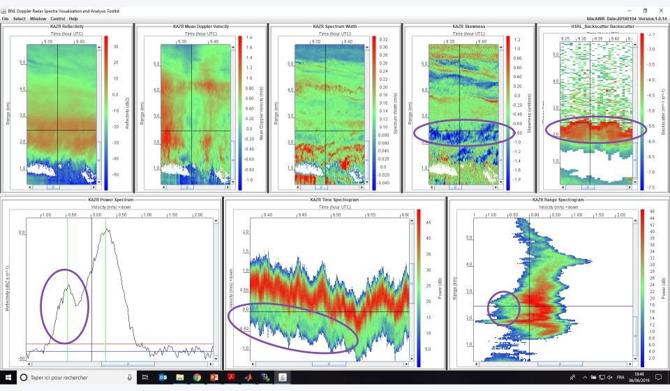
Clearly, the high  $DWR_{KaW}$  layer is associated with a long-lasting cloud liquid layer seen in the Doppler spectra and by the lidar
