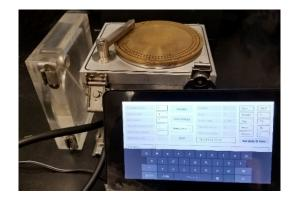
Time Resolved Aerosol Collector (TRAC) <u>Time per sample: 7 min</u>
